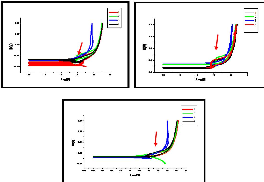
**Figure 5: Cyclic Anodic Polarization Curves For (A, B), 1, 2 MI Fire Steel Fiber and (C) 1ml Withdraw Steel Fiber in 3.5%NaCl Solution at 25C<sup>0</sup>.**
