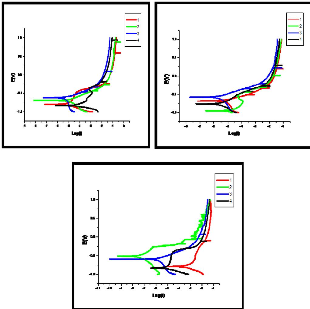
**Figure.2: Anodic and Cathodic Polarization Curves**
