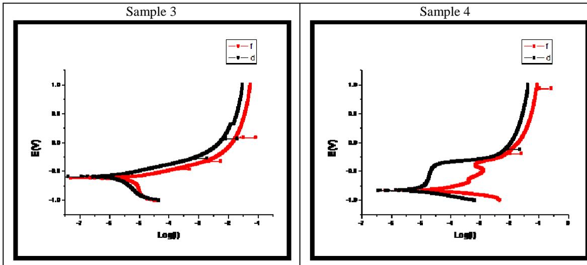
Figure.4: Comparison between Fire (F) and Drawn (D) Steel Fiber Samples at 25C<sup>0</sup>
