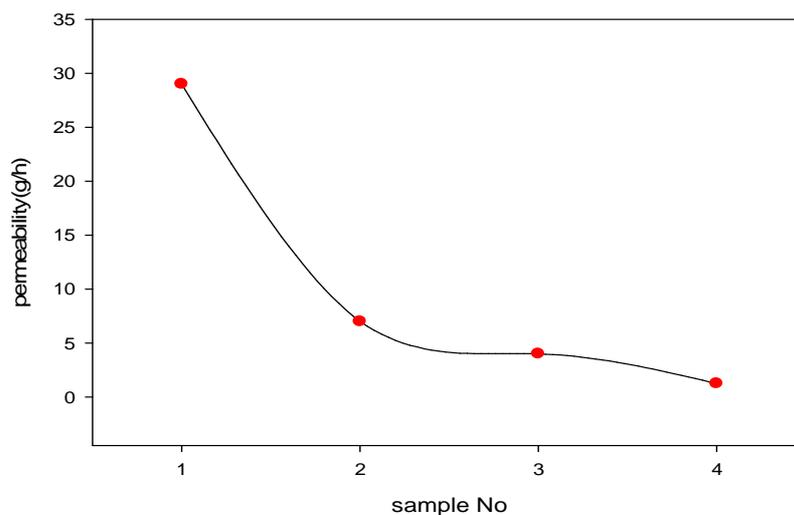
**Figure 1: Permeability of Steel Fiber Reinforced Concrete**
