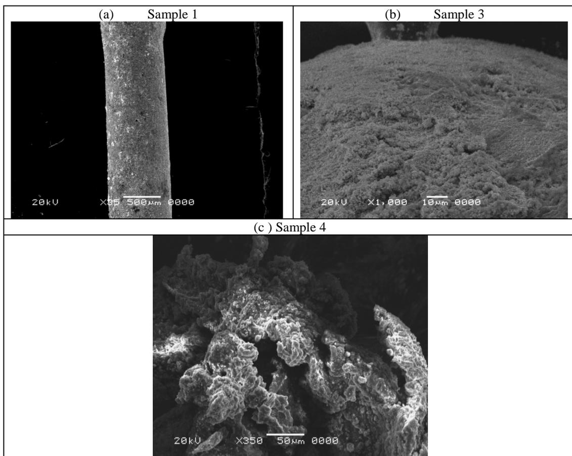
**Figure.6: Surface Morphology of Three Fire Steel Fiber Samples In 3.5% NaCl Solution.**
