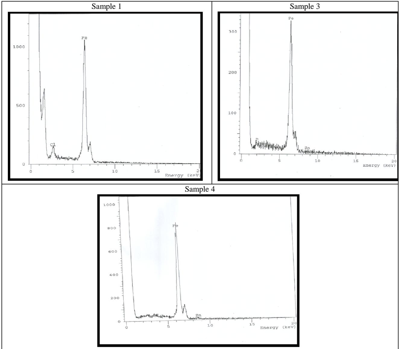
**Figure 9: EDAX Spectra of Draw Steel Fiber In 3.5% NaCl Solution.**
