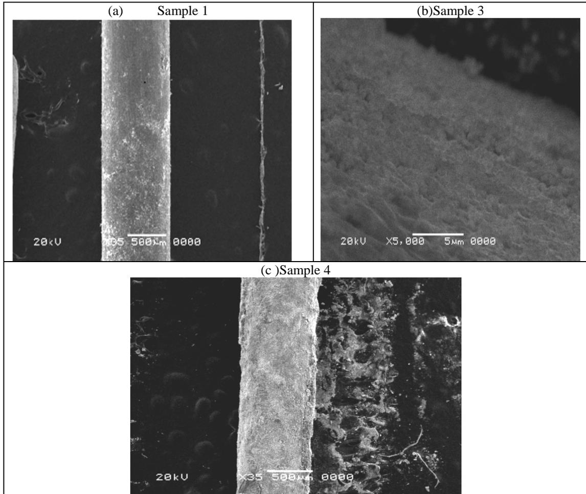
**Figure.7: Surface Morphology of Three Samples of Steel Fiber (Withdraw) In 3.5% NaCl Solution.**
